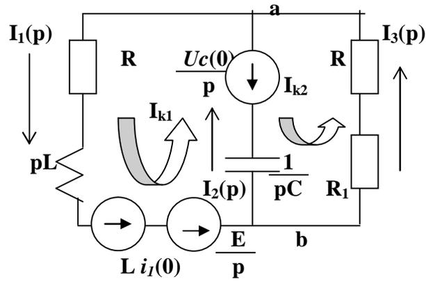
$$\left. \begin{aligned} I_{k1} \left( R + pL + \frac{1}{pC} \right) - \frac{I_{k2}}{pC} &= Li_I(0) + \frac{E - U_c(0)}{p} \\ -\frac{I_{k1}}{pC} + I_{k2} \left( R + R_1 + \frac{1}{pC} \right) &= \frac{U_c(0)}{p} \end{aligned} \right\}$$
